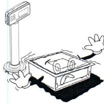
By adjusting 4 corners of the scale, set the scale even using the built in scale leveling indicator.
