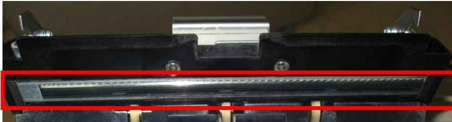
CIS sensor surface (glass)
